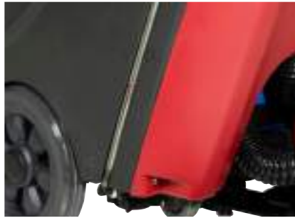
Water level indicator with volume visible on tank
